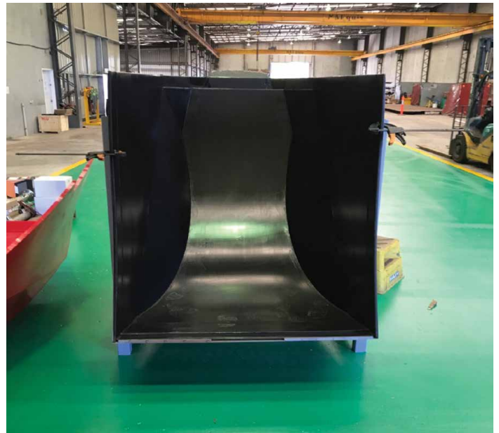
Fig. 2 - Typical Polyurethane rubber liner weighing ca. 200kg.
