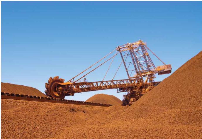
Fig. 1 - Typical Sandvik 12,000 tph bucket-wheel reclaimer.
