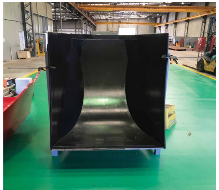
Fig. 2 - Typical Polyurethane rubber liner weighing ca. 200kg.
