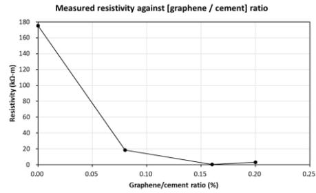
Figure 5 Fig. Electrical Resistivity (kΩm) of cement containing PureGRAPH<sup>®</sup> graphene additives.
