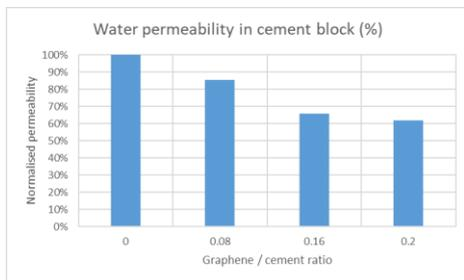
Figure 4 Fig. Water permeability of cement pastes containing PureGRAPH<sup>®</sup> graphene additive
