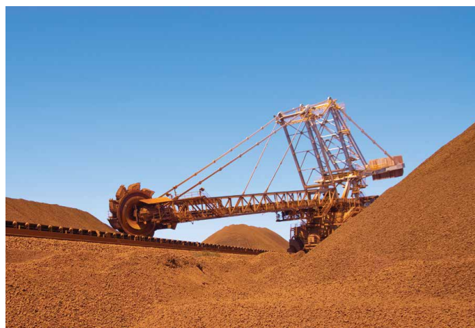
Fig. 1 - Typical Sandvik 12,000 tph bucket-wheel reclaimer.
