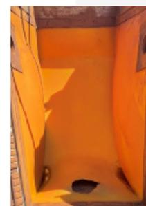
Fig. 3.2 Standard PU Liner after field trial
