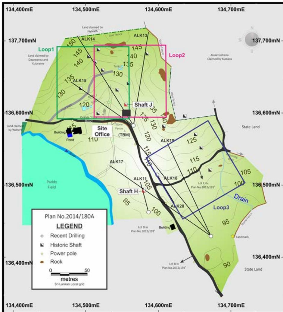
Figure 7: Aluketiya project site plan with Shafts H and J and exploration drill hole traces and transmitter loop locations
