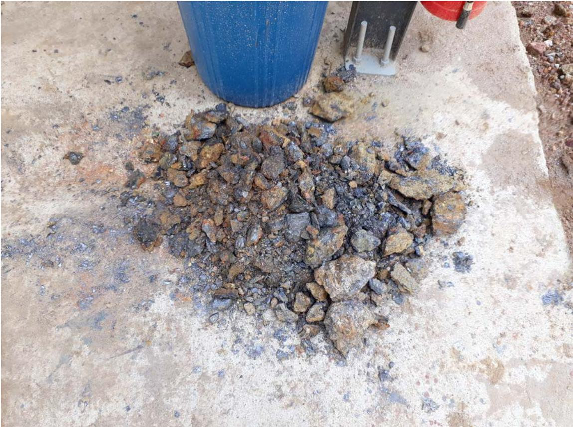
Figure 4: Weathered vein graphite extracted from Shaft J as it is being sunk
