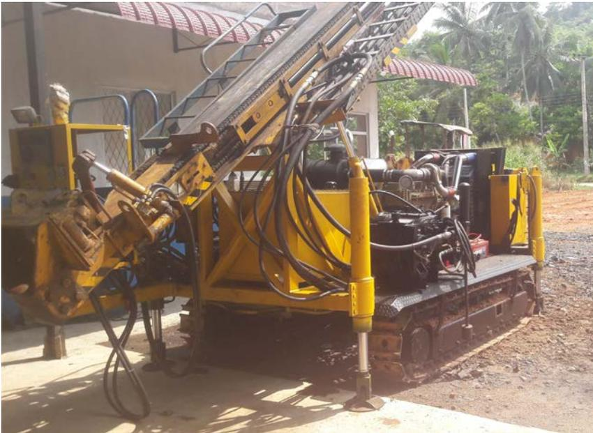
Re-powered XT400THD Drilling Rig
