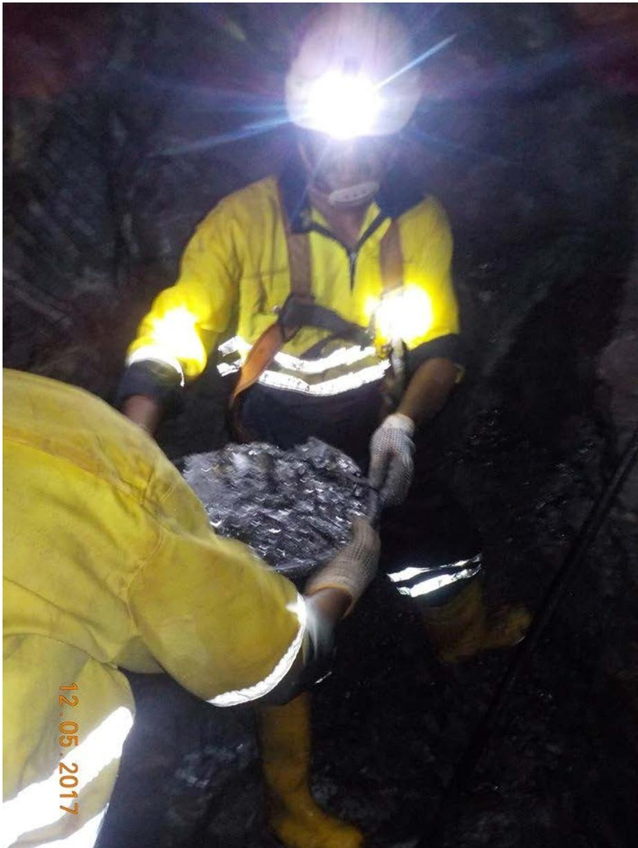
Shaft H vein graphite ore being extracted
