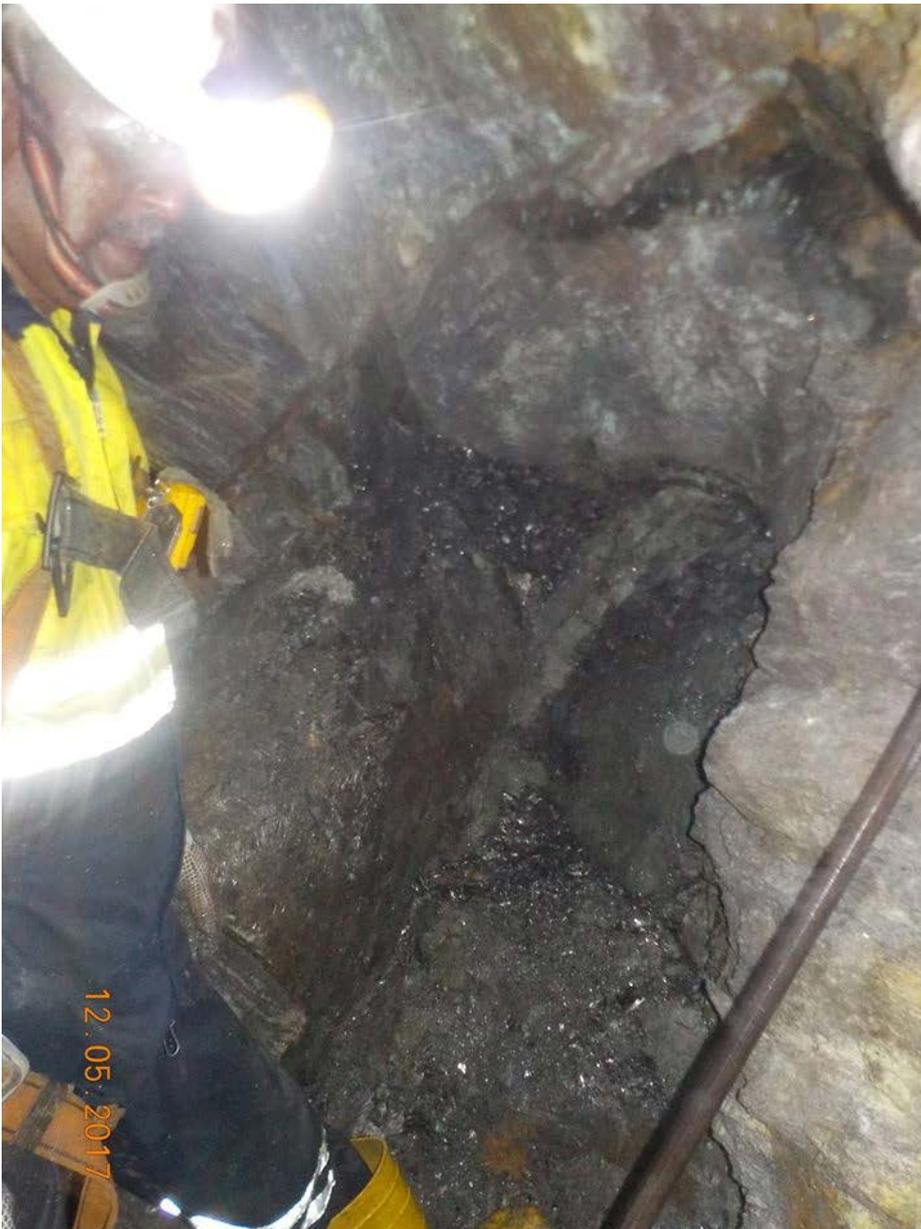
Graphite vein in Shaft H level drive being mined
