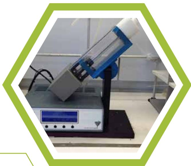
Laboratory scale Vortex Fluidic Device
