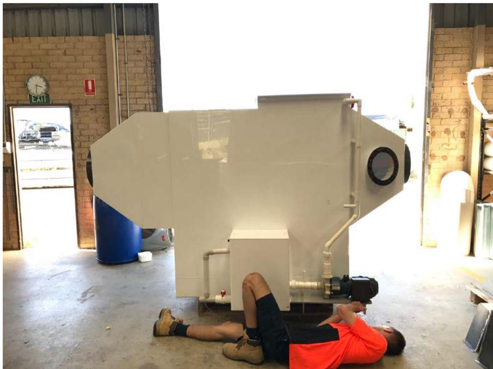
Figure 4: Cross Flow Scrubber ready for installation
