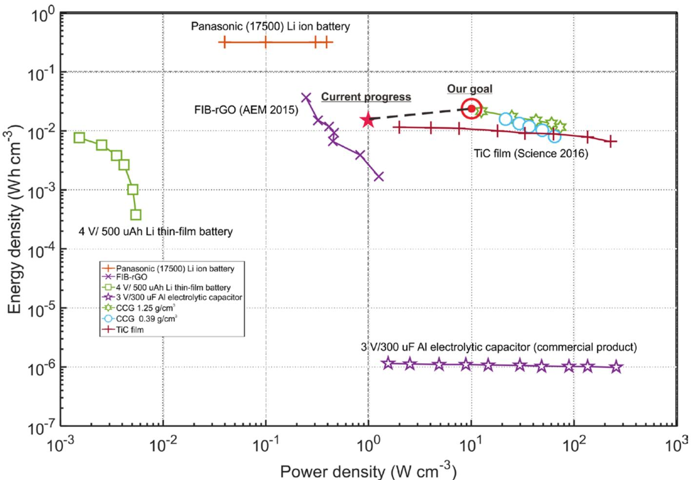
Figure 1: Ragone Plot demonstrating the progress of the BEST™ Battery development toward its goal
