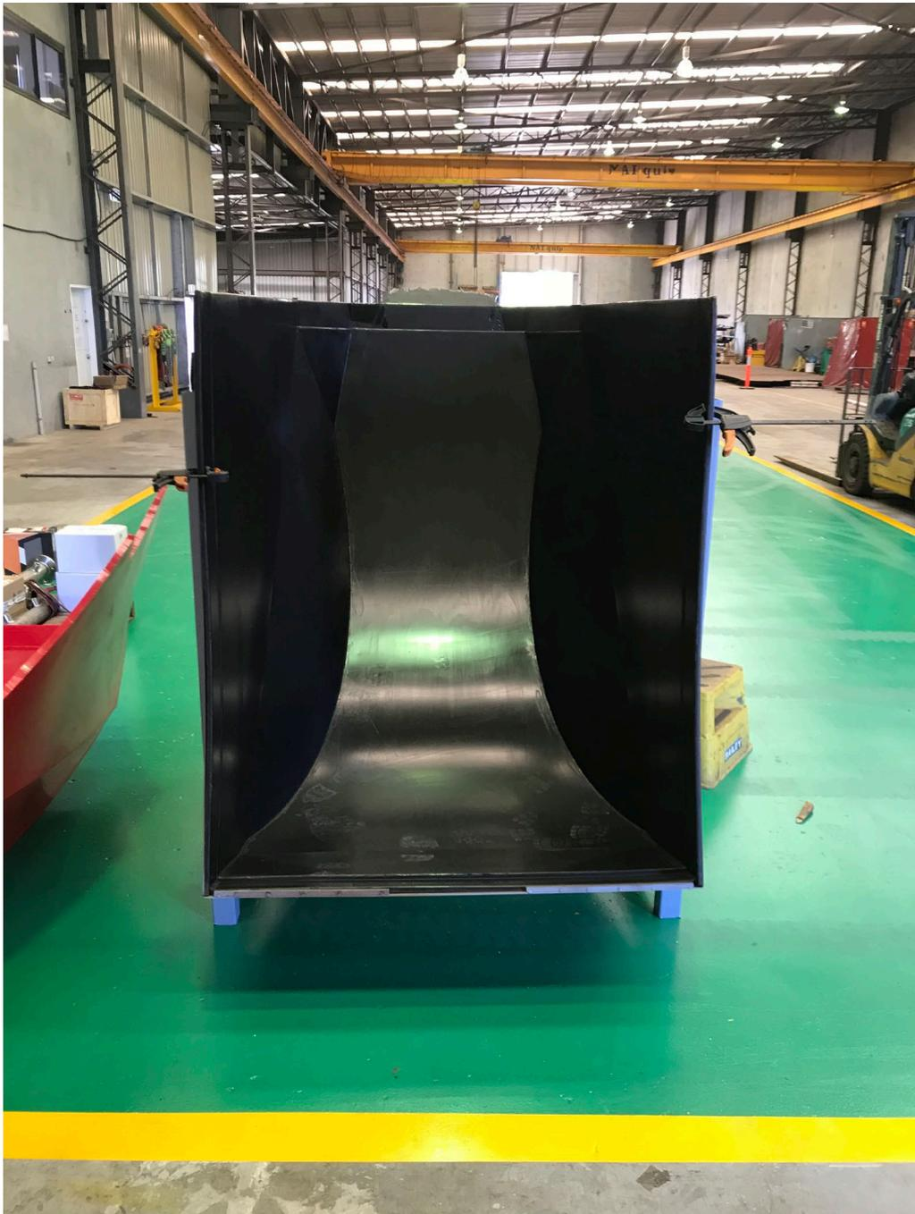
The reclaimer bucket liner has 200kg of polyurethane and is strengthened by PureGRAPH™ 20
