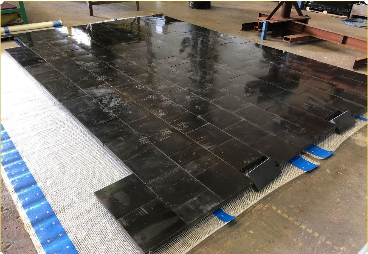
Armour-GRAPH™ panels being assembled at newGen's facility
