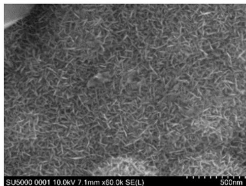
**Fig. 1: Metal Oxide decorated graphene surface – crystalline metal oxide nanostructures grown directly onto the graphene platelet. Considered to be an ideal structure for capacitance and catalysis.**
