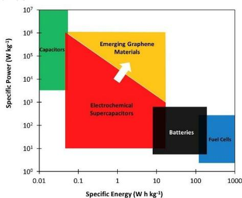
**Fig. 1: Ragone diagram comparing the performance of supercapacitors with chemical batteries and showing the opportunity for graphene.**
