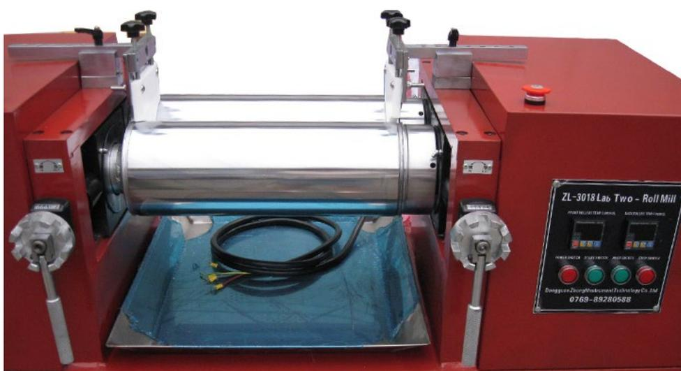
*Figure 1, Lab scale two roll mill*
