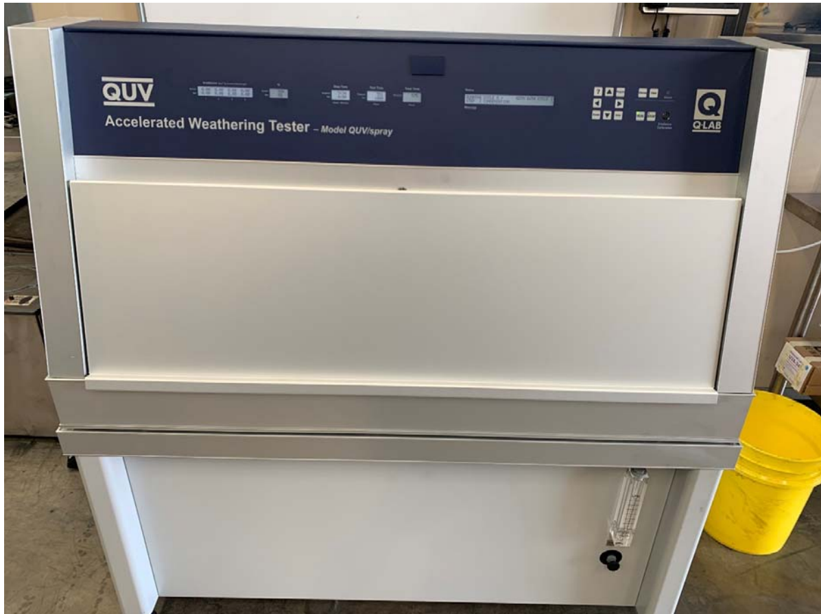
FGR's Accelerated Weathering Tester running a 1,000 hour test to ASTM G154 standards for composite materials.
