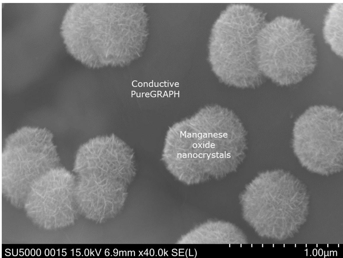
**Fig. 1 Manganese (IV) oxide nanostructures grown directly onto a graphene scaffold.**
